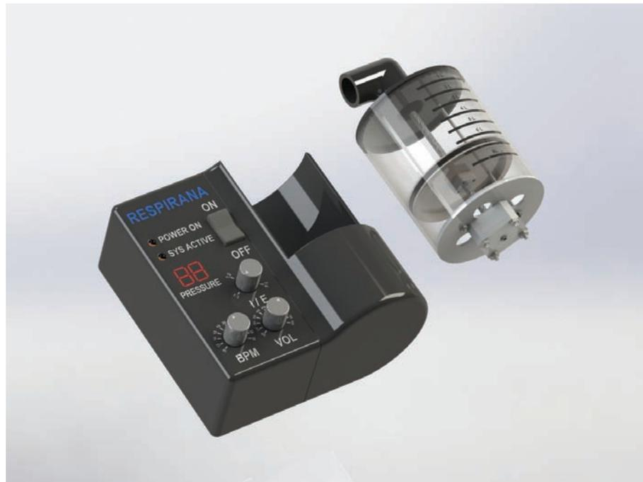
Designers used the BVM bag in a novel fashion and developed a piston design to deliver positive pressure. This preserves the BVM bag from being squeezed too many times and allows for more precise ventilator settings to be utilized.
