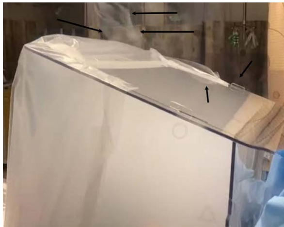
Fig. 3. Vapor egress (arrows) from the unsealed edge of the interlocking box. The video in the Supplemental Digital Content ( http://links.lww.com/ALN/C502 ) provides additional visualization of vapor egress.
