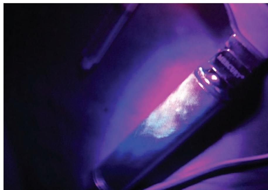
**Figure 3:** Image showing contamination of a laryngoscope handle on the anesthesia machine after use during a simulated induction on a mannequin with fluorescent gel placed in the mouth as a proxy for oral microorganisms.
