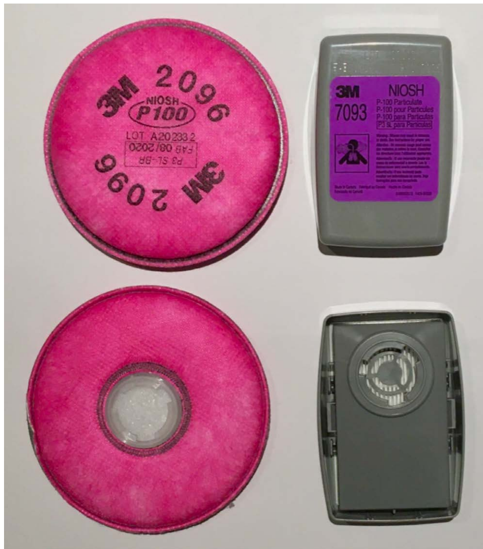
Fig. 2. Examples of elastomeric respirator filters. The outer facing side of the filters is shown in the upper photos , and the side of the filters that attaches to the respirator is shown in the lower photos . Both filters are P100 (equivalent to high-efficiency particulate air). The filtering material of the left filter is exposed, while the filtering material of the right filter is completely enclosed in plastic. The right filters are also shown mounted on an elastomeric respirator in fig. 1C.
