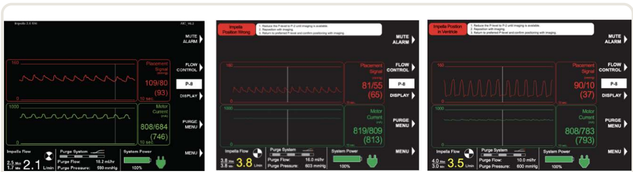
Fig. 2. Placement screen on the Automated Impella Controller. Placement screens generated by a fluid-filled pressure lumen (Impella 2.5 and CP) are shown. ( Left ) The transvalvular heart pump is appropriately positioned and shows an aortic waveform in the placement signal and a pulsatile motor current. ( Middle ) The blood inlet and outlet areas are both in the aorta (aortic waveform placement signal, flat motor current). ( Right ) Both the inlet and outlet areas are in the ventricle (ventricular waveform placement signal, flat motor current). Please see figure A1 for placement screens generated by a differential pressure sensor. Adapted and reproduced with permission from Abiomed Inc. (USA).
