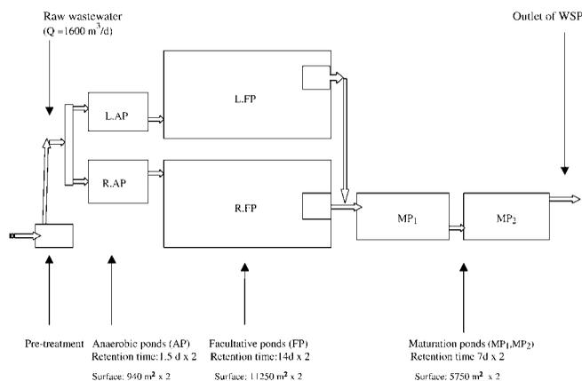
Figure 1 | Schematic flow diagram for Boujaâd WSPs.
