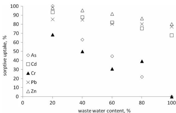
Figure 1 | Sorptive uptake from batch experiments for selected heavy metals and metalloids.
