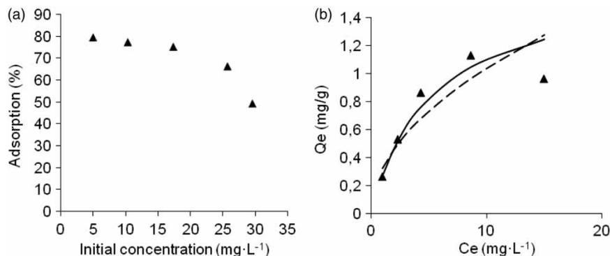
**Figure 3** | Percentage sorption of TNT to pine bark at various initial concentrations (a) and Langmuir (solid line) and Freundlich (dotted line) model fits for TNT isotherm data (b).
