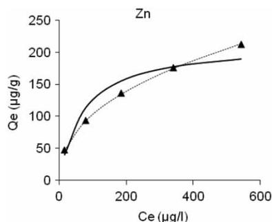
**Figure 2** | Langmuir isotherm (solid line), Freundlich isotherm (dotted line) fitting for adsorption of Zn data (▲) to pine bark.
