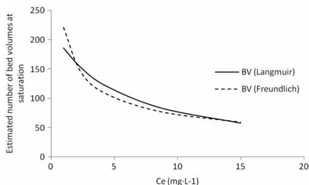
**Figure 4** | Estimated number of bed volumes (BV) to TNT saturation of a packed bed reactor at different equilibrium (or influent) TNT concentrations based on Langmuir and Freundlich isotherm models.
