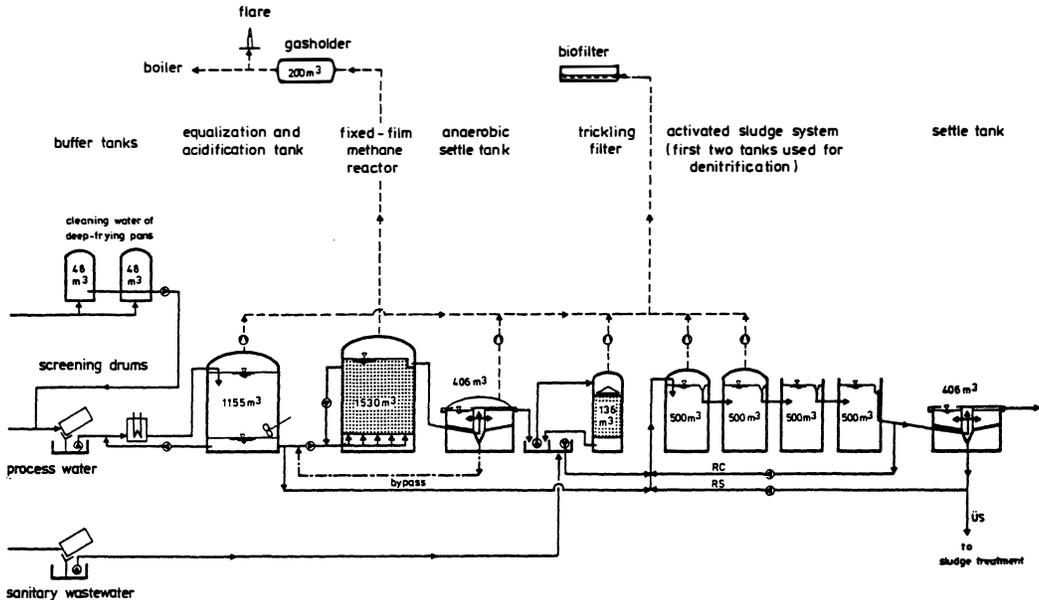
Fig. 1. Flow diagram of the anaerobic-aerobic wastewater treatment plant of a potato chips factory
