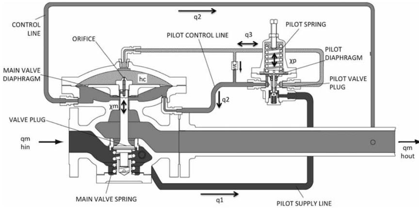
Figure 3 | The PRV scheme and governing flows.
