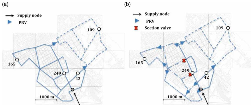
**Figure 5** | Position of the PRVs and closed pipes on network mains: Scenario A (a) and Scenario B (b). The blue lines define the boundaries of the PMAs. Please refer to the online version of this paper to see this figure in colour: <http://www.iwaponline.com/jh/toc.htm>.
