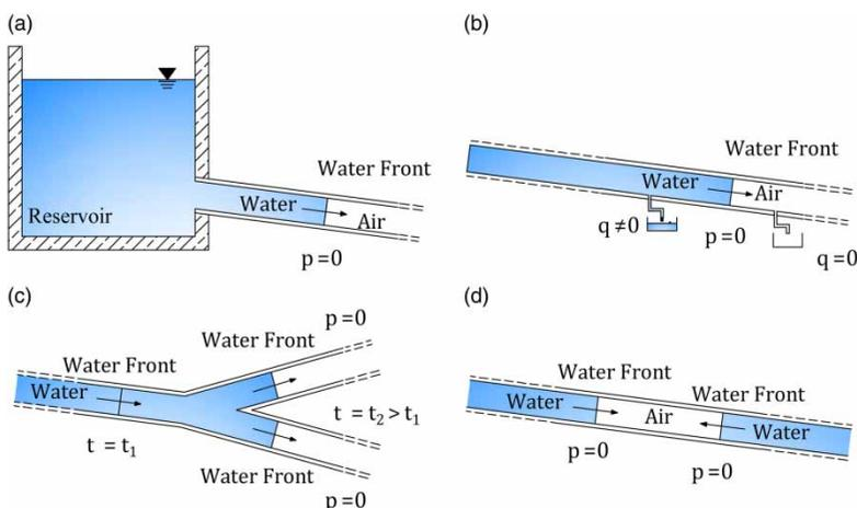
**Figure 1** | Hydraulic schematics of the network filling process: (a) initial phase of water front propagation; (b) water front reaches a user connection; (c) water front reaches the end of the pipeline; (d) two water fronts proceed inside the pipe in opposite directions.
