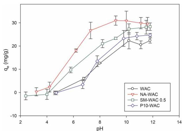
**Figure 3** | Effect of equilibrium pH on the adsorption of TMAH on WAC and modified WACs ( $C_0$ :  $20 \pm 2$  mg/L (a),  $C_0$ :  $500 \pm 50$  mg/L (b), adsorbent dose: 4 g/L, reaction time: 24 hours).
