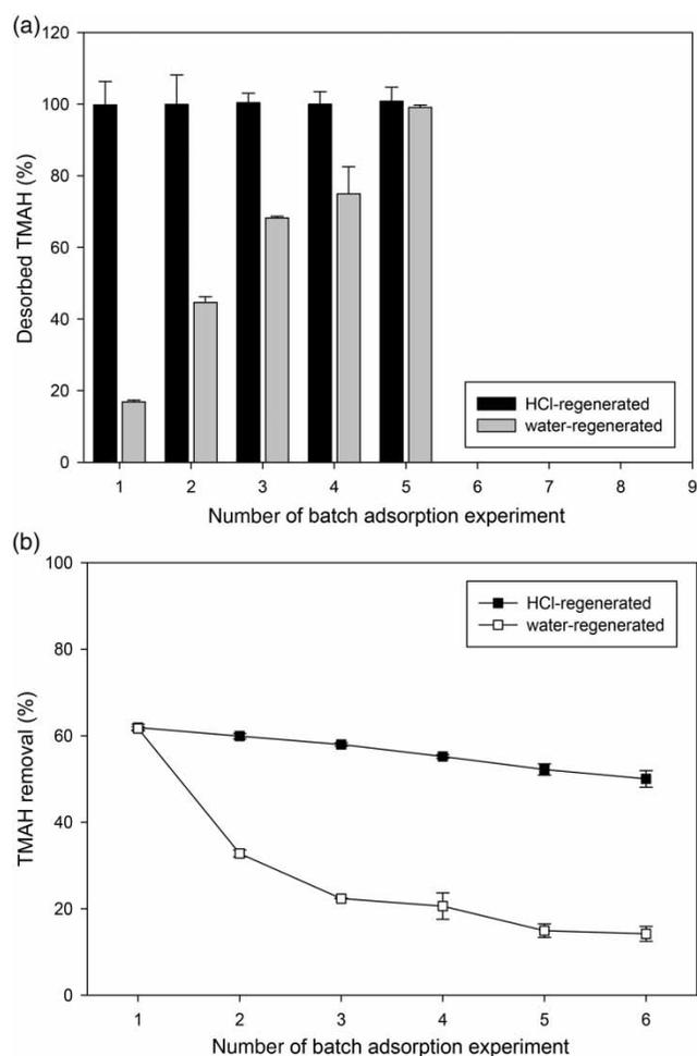
**Figure 4** | (a) Regeneration of NA-WAC by 0.1 N HCl and water ( $C_0$ :  $50 \pm 5$  mg/L, adsorbent dose: 4 g/L, pH:  $11.8 \pm 0.2$ , reaction time: 24 hours). (b) Batch adsorption cycles of NA-WAC ( $C_0$ :  $50 \pm 5$  mg/L, adsorbent dose: 4 g/L, pH:  $11.8 \pm 0.2$ , reaction time: 24 hours).
