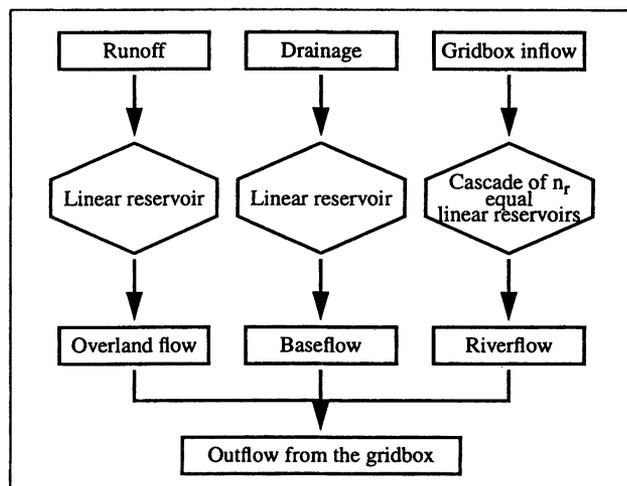
Fig. 1. Structure of the HD model.
