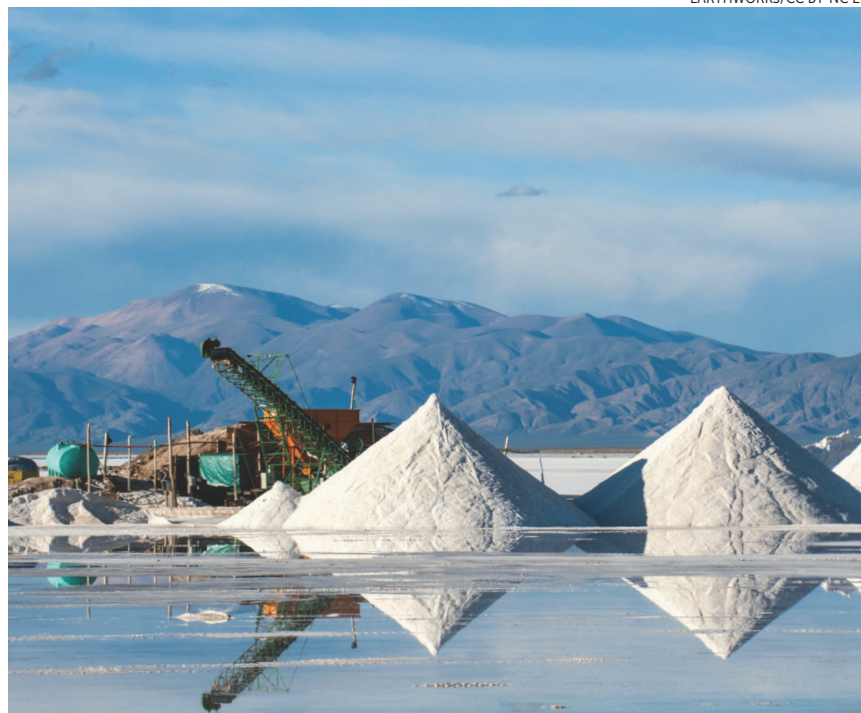
A LITHIUM BRINE operation at the Salinas Grandes salt flats in Argentina. Around 30% of the world supply of lithium is from South American brines.
