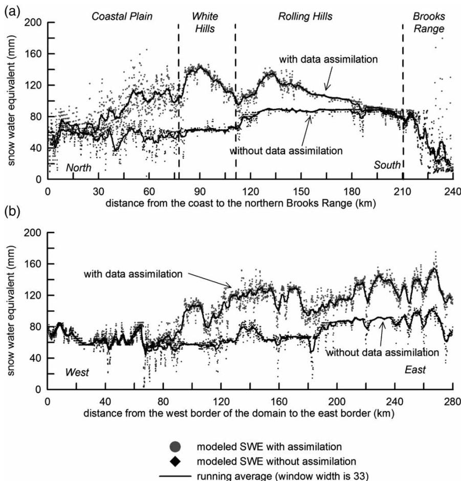
**Figure 8** | Comparison of model SWE with and without assimilation of observational data. Modeled SWE was extracted for 21 April 2009, along the (a) north-south and (b) west-east bands. Location of these bands is shown in Figure 7(b). Each band is 1 km wide and includes 10 grid cells. Grey dots indicate averaged SWE across the band; corresponding lines show running average.
