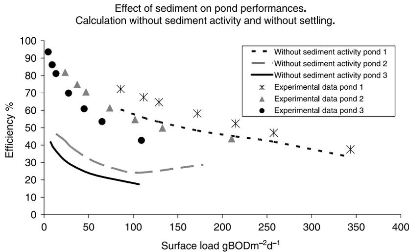
Figure 3 Efficiencies of aerated lagoons in series. Comparison to literature data
