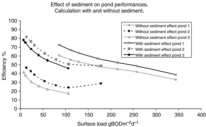
Figure 4 Effect of sediments. Comparison with the 'chemostat' model
