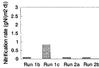
**Figure 11** Nitrification rate of the sloughed biofilm by water spray
