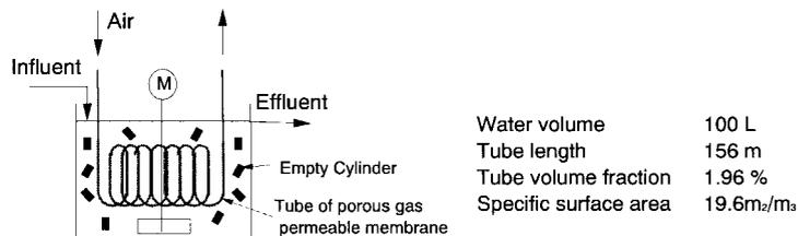
**Figure 1** Tube reactor
