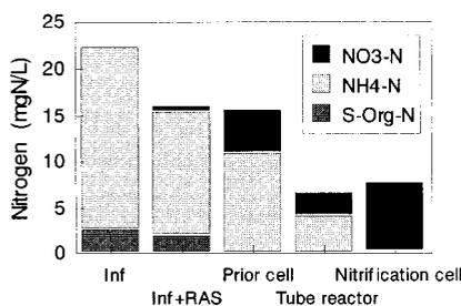
**Figure 4** Change of nitrogen concentration along flow direction in Run 1b (after 69d)
