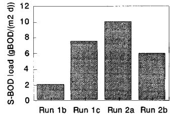
**Figure 12** Soluble organic load to tube surface
