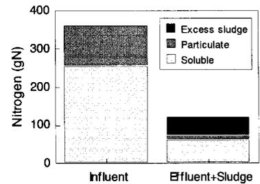
**Figure 8** Nitrogen balance in Run 1c
