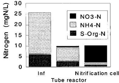
**Figure 7** Change of nitrogen concentration along flow direction in Run 2a
