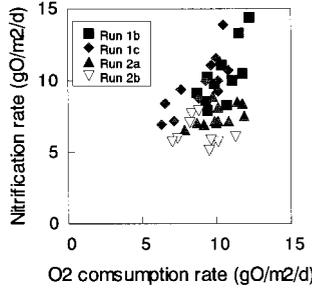
**Figure 13** Relationship between  $O_2$  consumption rate and nitrification rate
