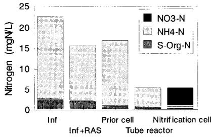
**Figure 5** Change of nitrogen concentration along flow direction in Run 1c
