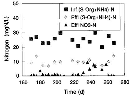
**Figure 6** Change of nitrogen concentration in Run 2
