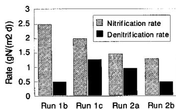
**Figure 9** Nitrification and denitrification rate of the tube before water spray
