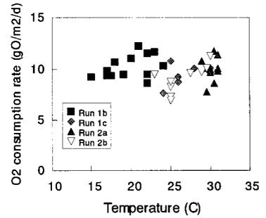
**Figure 14**  $O_2$  consumption rate of tube reactor in each Run
