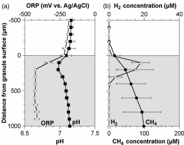
**Figure 2** | Concentration profiles of pH and ORP (a), and CH<sub>4</sub> and H<sub>2</sub> (b) in the anaerobic granule. The profiles are average values ( $n = 3$ ) and error bars represent the standard deviations of triplicate measurements. Zero on the vertical axis corresponds to the surface of the granule.
