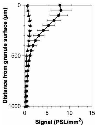
**Figure 5** | Vertical distribution of local scintillation signals in granules incubated with sodium [<sup>1-14</sup>C]propionate (▲) and D-[U-<sup>14</sup>C]glucose (●) determined from beta microimaging data (Figure 4). The profiles are average values ( $n = 6$ ) and error bars represent the standard deviations.
