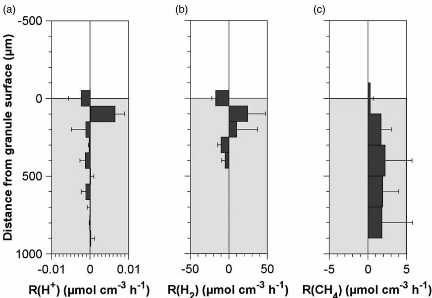
**Figure 3** | Spatial distribution and magnitude of the net volumetric production rates of acid (i.e. H<sup>+</sup>) (a), H<sub>2</sub> (b) and CH<sub>4</sub> (c). The rates were calculated based on the corresponding concentration profiles shown in Figure 2. Negative values indicate consumption rates. Zero on the vertical axis corresponds to the surface of the granule.
