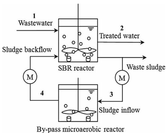
Figure 1 | Schematic diagram of the five experimental systems. (Note: M represents peristaltic pump, numbers 1–4 represent sampling points.)
