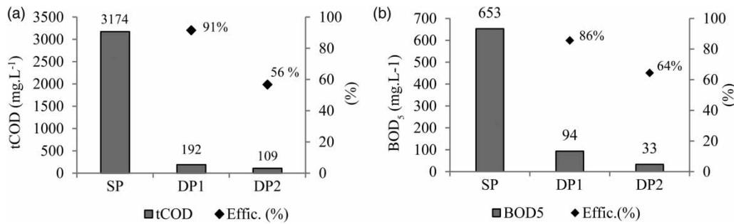
**Figure 3** | Mean values for the BOD<sub>5</sub> and tCOD concentration throughout the duckweed pond system and the average removal efficiency (SP = storage pond influent; DP1 and DP2 = duckweed pond 1 and 2).
