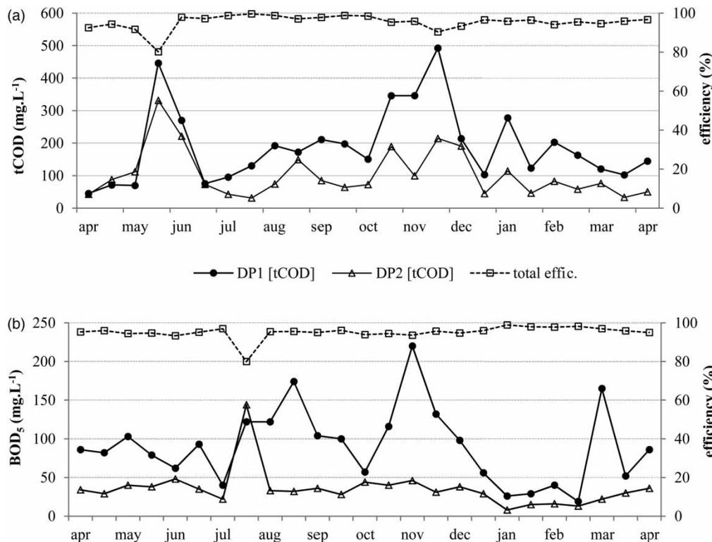
**Figure 4** | tCOD (a) and BOD<sub>5</sub> (b) concentration and total efficiency over the monitoring period (DP1 and DP 2 = duckweed pond 1 and 2).
