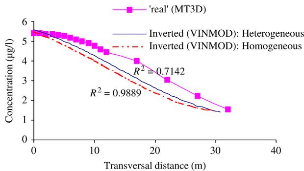
Figure 15 | Inverted concentration distributions under heterogeneous and simplified homogeneous cases compared with the “real” concentration distribution.
