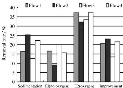
Figure 5 Total COD removal efficiency of each flow
