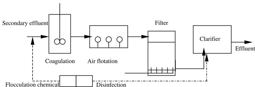
Figure 2 Flow scheme of 3200 m<sup>3</sup>/d advanced treatment process
