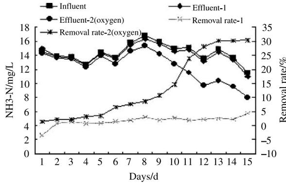
Figure 3 Ammonia nitrogen removal rate at the startup
