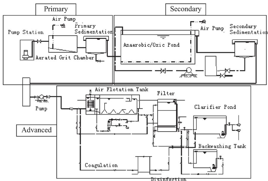
**Figure 1** Conventional secondary wastewater treatment and advanced clarification in Harbin Wenchang WWTP
