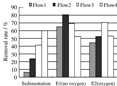
**Figure 9** SS removal efficiency of each unit building
