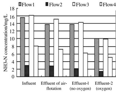
**Figure 6** NH<sub>3</sub>-N variation of each flow
