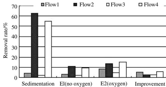
**Figure 8** TP removal efficiency of each unit building
