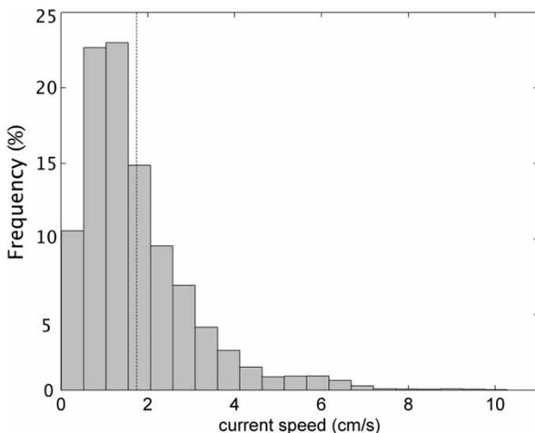
**Figure 7** | Normalised histogram of current speeds from the inshore site over the deployment period. These speeds are 1 minute averages from the 60 cm range above the sediment. The mean current speed of  $1.75 \text{ cm s}^{-1}$  is shown as the vertical dashed line.
