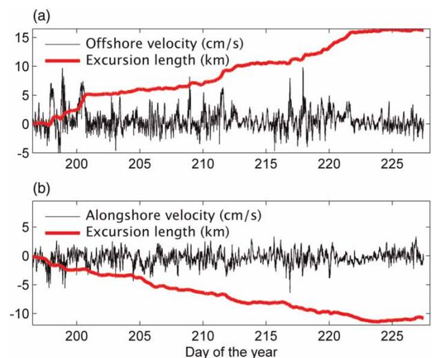
**Figure 5** | Velocity (black) and excursion length,  $L(t)$  (red) at the inshore site. In (a) velocity and excursion are positive in the east direction, in (b) velocity and excursion length are positive in the north direction. The y-axis in each subfigure is 21.5 units of either velocity in  $\text{cm s}^{-1}$ , or distance in km. The full colour version of this figure can be found online at <http://www.iwaponline.com/wqrj/toc.htm>.
