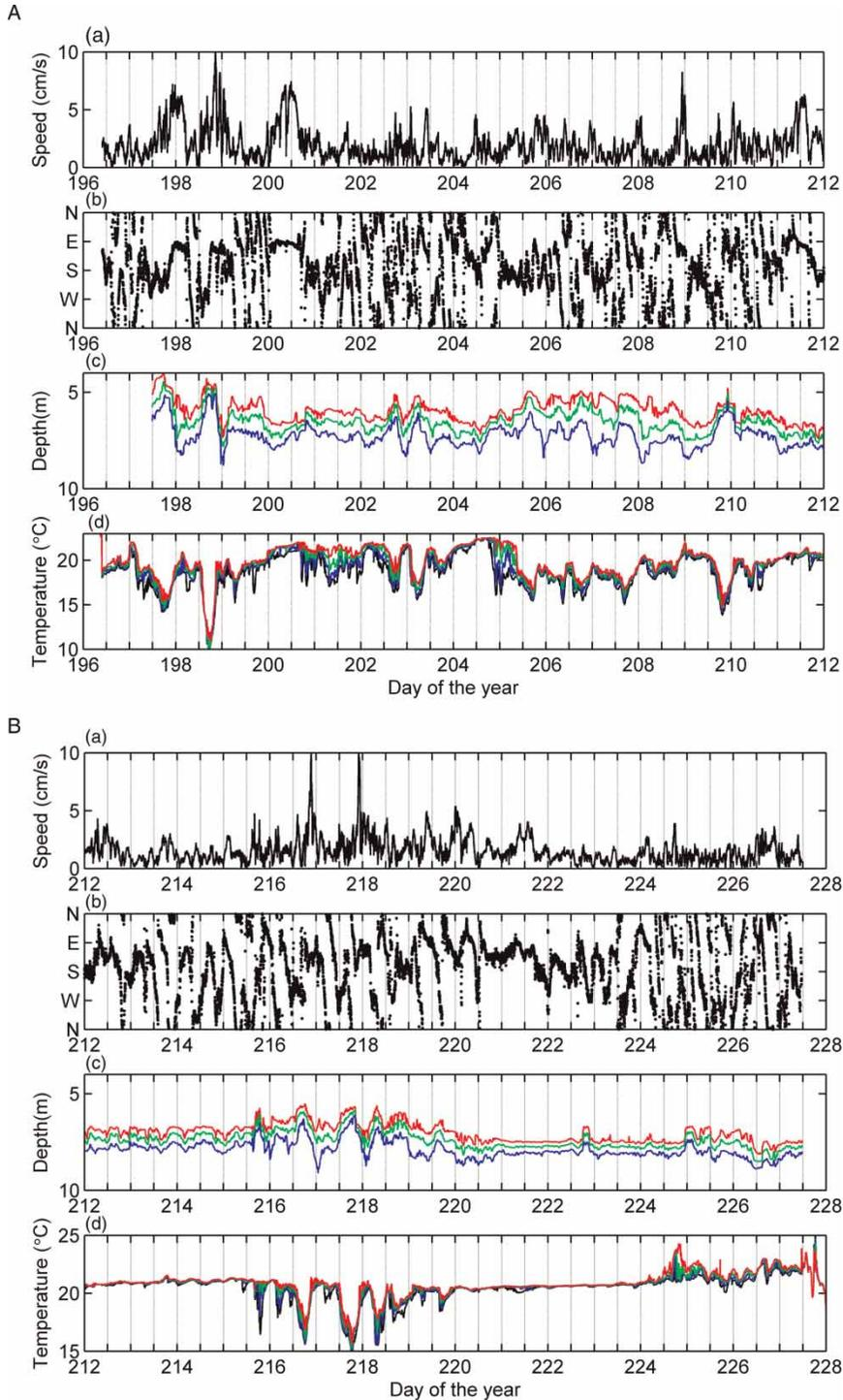
**Figure 3** | (a) Current speed at the inshore site, (b) current direction at the inshore site, (c) isotherms at the offshore site with the 15.5 °C isotherm in blue, 17.5 °C in green and 19 °C in red, and (d) isodepths (temperature at a fixed depth) at the inshore site, 0.3 m (black), 0.6 m (blue), 0.9 m (green) and 1.2 m (red) above the sediment. The full colour version of this figure can be found online at <http://www.iwaponline.com/wqrj/toc.htm>.
