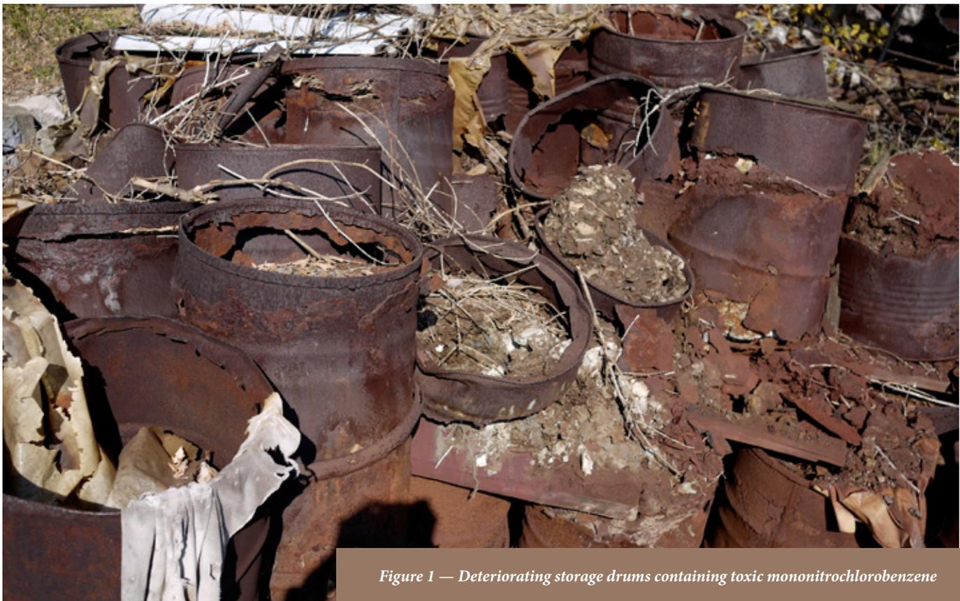
Figure 1 — Deteriorating storage drums containing toxic mononitrochlorobenzene
