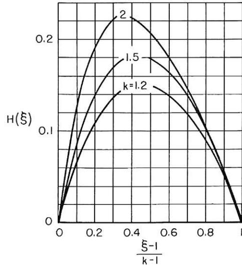
Fig. 7 Function for temperature rise owing to viscous shear for steady rotational motion, after Schlichting [7]
