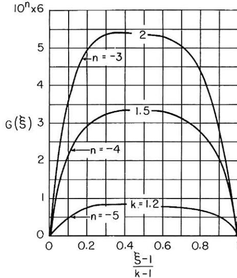
Fig. 6 Function for temperature rise owing to viscous shear for steady longitudinal flow
