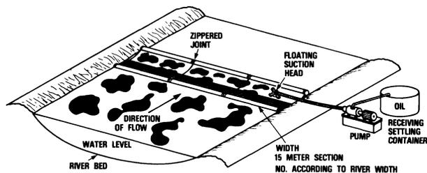
Figure 2. Deployed boom
