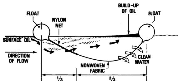
Figure 1. Cross section of boom
