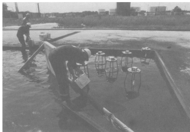
Figure 2. One barrel of light crude oil was poured into an open fire test basin to test for benzene vapor.
