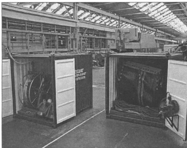
Figure 1. Compact containerized offshore containment and recovery package.
