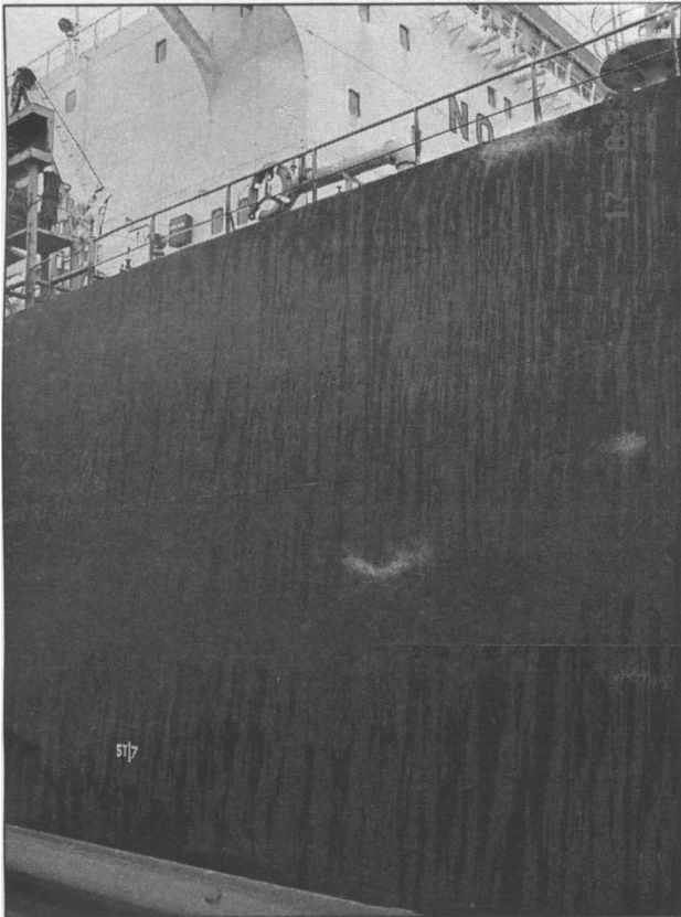
Figure 2. Starboard side looking aft of the M/V GENMAR HECTOR. Note streaks of oil on the hull and superstructure.
