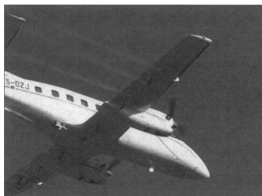
FIG.4 - VIEW FROM BELOW OF THE WING MOUNTED SPRAY BOOMS IN ACTION.
