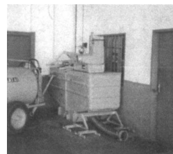
FIG.3 - THE SPECIALLY DESIGNED DISPERSANT TANK AND PUMP UNIT.
