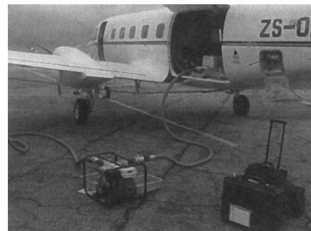
FIG.9 - THE RESPONSE CREW PRACTICE LOADING THE DISPERSANT INTO THE TANK.
