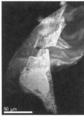
FIGURE 3. FLAKE OMA HAVE A MEMBRANE-LIKE STRUCTURE. THE FLUORESCING CHARACTER OF THE OMA SUGGESTS THE PRESENCE OF OIL.
