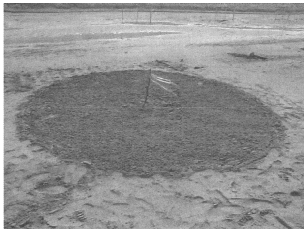
FIGURE 3. TEST PLOT FOR TREATMENT OF OIL CONTAMINATION AT THE KHOR AL-MUFATEH SITE.
