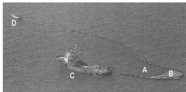
FIGURE 1: A NOFO SYSTEM; A-OIL AGGREGATING AREA, B- OIL COLLECTED IN THE BOOM, C-OIL RECOVERY VESSEL, D- TOWBOAT.
