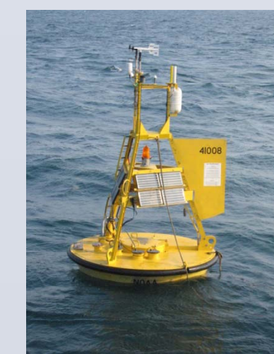
Example of data buoy from which students derive information on wave heights. Photo: PMEL/NOAA
