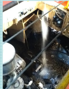
Solidifying agent being applied to engine room
