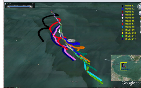
Figure 4. Twelve oil spill predictions (GNOME) animated on Google Earth (Hou and Hodges, 2014). The different color dots denote different oil spill predictions based on different combinations of wind/tide/inflow hindcast/forecast. The whole movie about this particular event can be found here: http://www.youtube.com/watch?v=5yNlOK6wJ4
