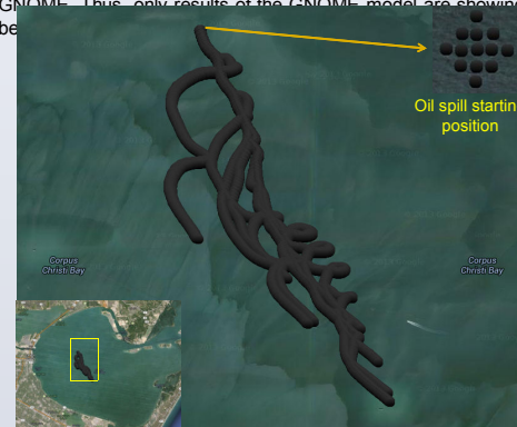
Figure 3. Twelve oil spill predictions (GNOME) visualized on Google Map (Hou and Hodges, 2014)
