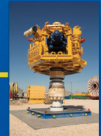
MWCC's 15k psi capping stack rerated to cap a well in temperatures up to 350 degrees Fahrenheit
