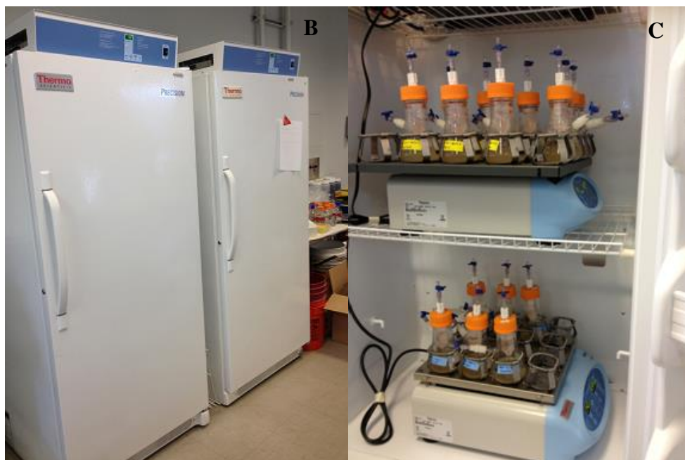
Figure 2. Experimental set-up: A) Schematic diagram of microcosms used to measure oil biodegradation; B) Incubators for controlled temperature; and C) Microcosm on shakers with a rotational speed of 140 rpm inside the incubators at the temperature of 15 \pm 0.5 °C.
