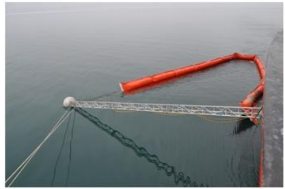
Figure 14. CG Spilled Oil Recovery System (SORS)
