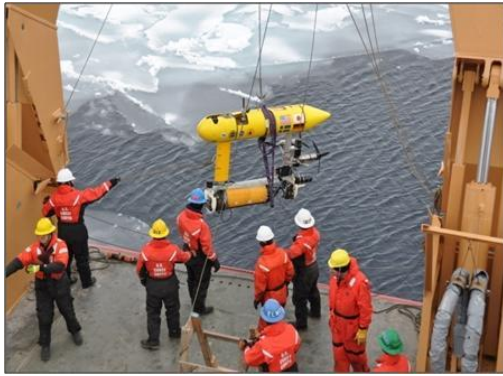
Figure 21 UUV Being Deployed
