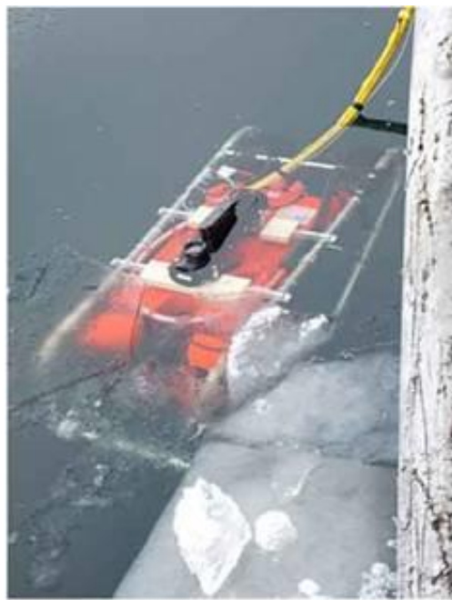
Figure 5. Remotely Operated Vehicle near ice
