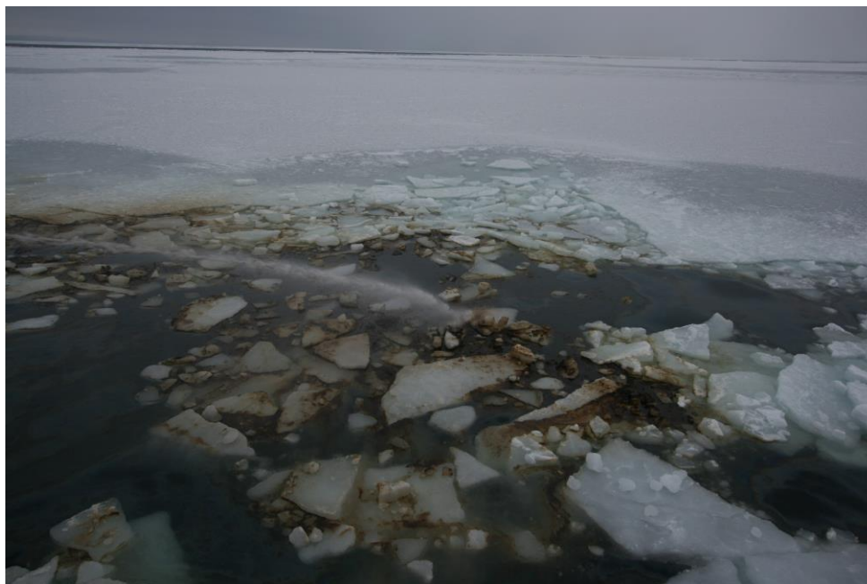
Figure 3. Addition of mineral fines to spilled oil.
