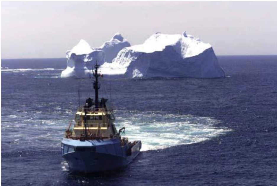
Figure 4. A vessel towing an iceberg away from an oil production site (Canadian Association of Petroleum Producers, n.d.).
