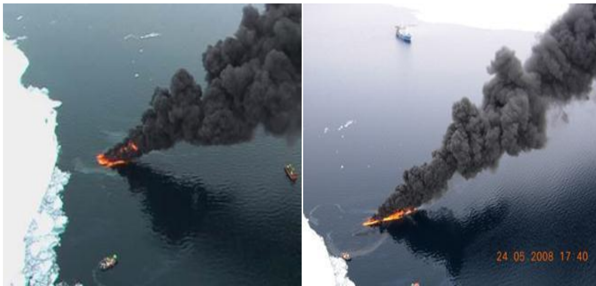
Figure 3. Burn of herded slick in Barents Sea ice lead (near start on left, near end on right)
