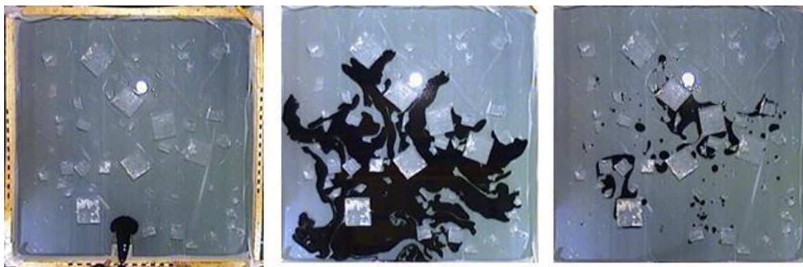
Figure 4. Testing of silicone-based herding agents at CRREL (far left shows oil release, centre shows oil spread at equilibrium, right shows contraction to new equilibrium after herder addition to water).
