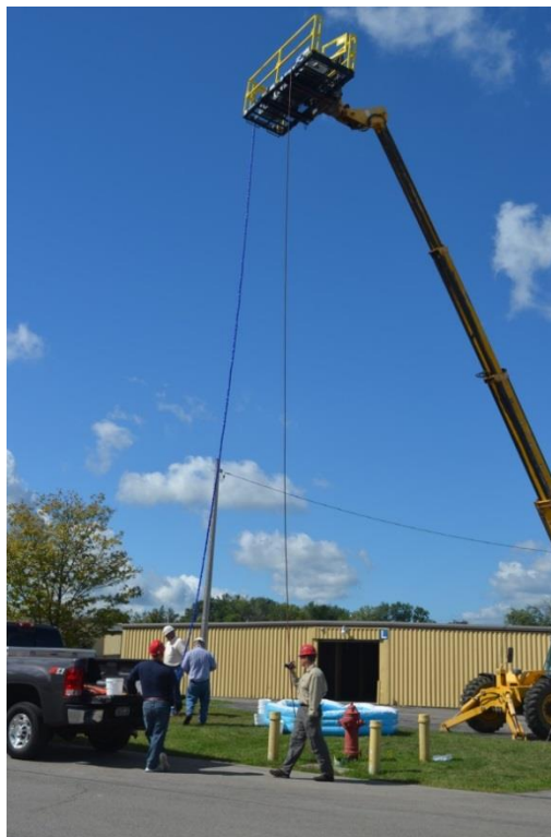
Figure 8. Applicator raised 46 feet above ground
