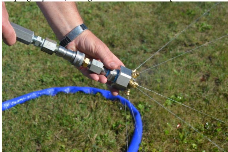
Figure 7. Applicator spray nozzle configuration.
