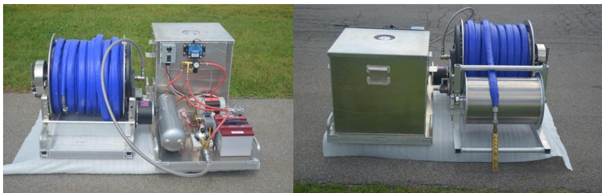
Figure 6. Mark I Helicopter Herder Application system
