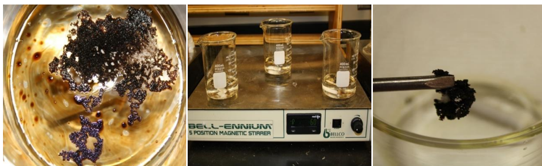
Fig. 1 Experimental setup showing (a) top view of oil slick and solidifier in a 400 mL beaker with fresh water; (b) triplicate samples mixing at 60 rpm for 30 min; (c) solidified product being removed with tweezers after contact time.
