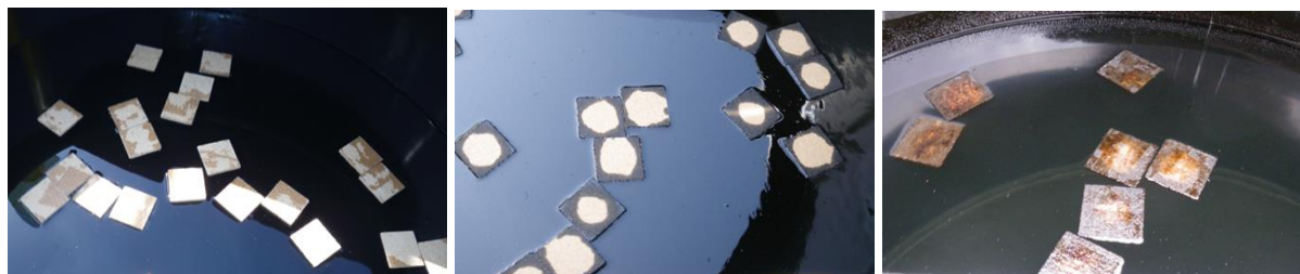
Figure 11 a-c: Cleaning process from beginning (a) and after 30 min (b) and 12 h (c) (Tank VII) After 12 hours the water surface was nearly clean (fig. 11 c). A detailed description of the mesocosm experiments can be found in Hähnel et al 2014 and Safanova et al 2014.
