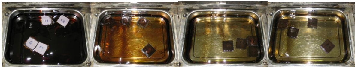
Figure 6: Cleaning process with binder after 5, 10, 15 and 90 min (crude oil)
