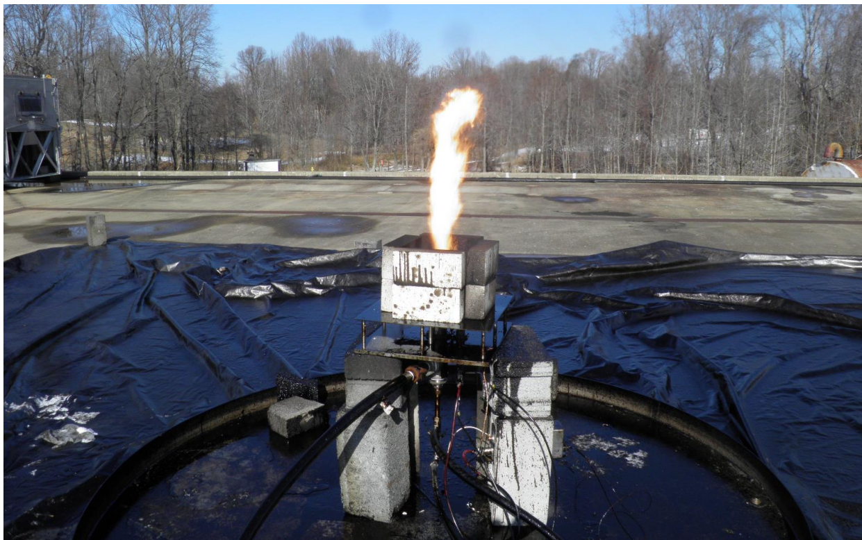
Figure 6. Burner mounted on pool fire burn pan catch basin and tarp to catch un-burned oil droplets: nozzle diameter = 7.04 mm, oil flow rate = 800 mL/min, and ALR = 0.5.
