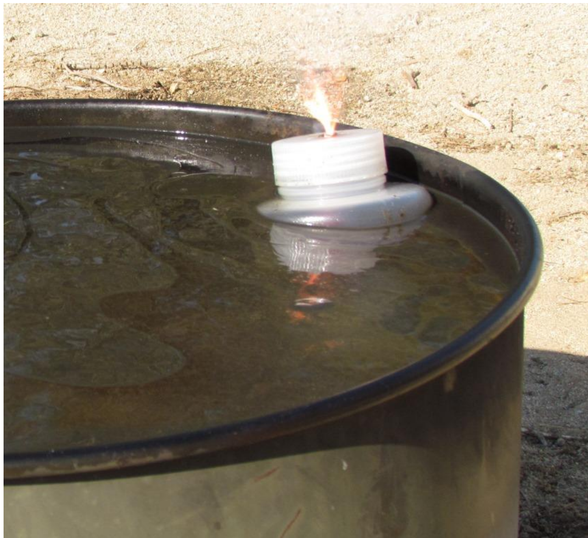
Figure 8. Initial flame from the initiator of the igniter (~2 min after injection).
