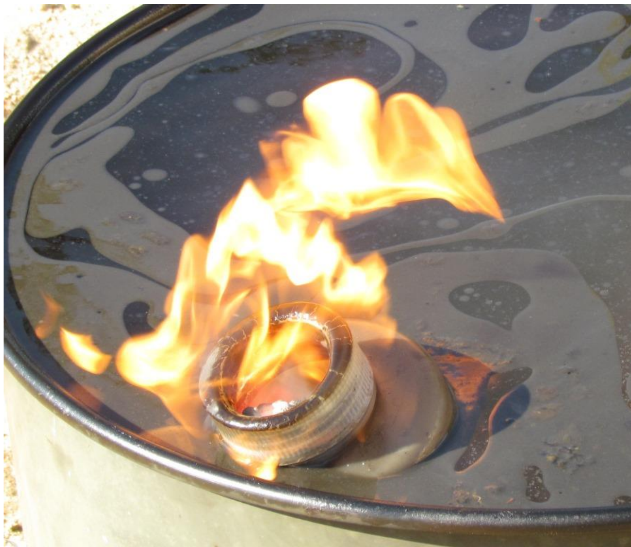
Figure 9. Initial burn-through of the lid of the igniter caused by the pyrotechnic booster (~3 min after injection).
