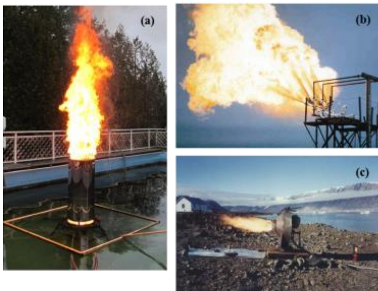
Figure 2. a) Chimney style burner, b) nozzle / flare style burner (courtesy of Zeeco Inc.), c) rotary cup burner (courtesy of SL Ross Inc.).
