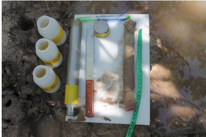
Figure 3. Collection of soil samples for hydrocarbon analysis. Samples were taken up to 22 cm and subdivided into 3 depths: 0-2cm, 10-12 and 20-22.
