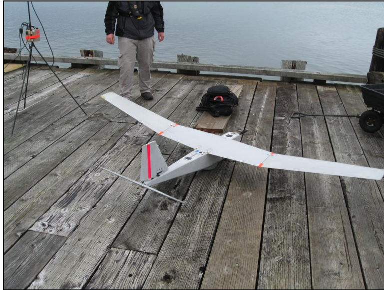
Figure 7: Puma UAS, assembled and ready for flight operations
