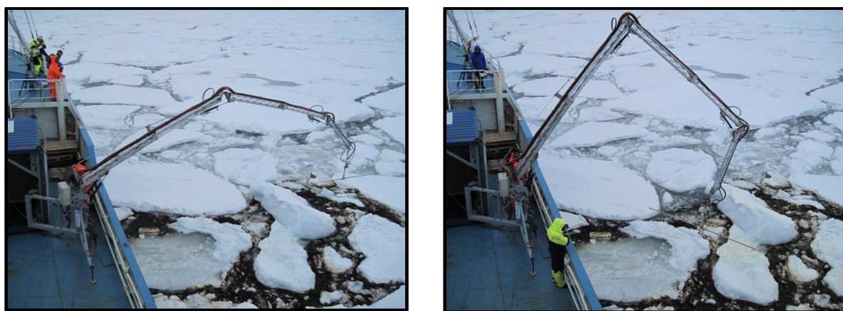
Figure 1. Prototype maneuverable, vessel-based dispersant spray system being used to apply dispersant onto oil spilled in ice (Photo Source: P. Daling).
