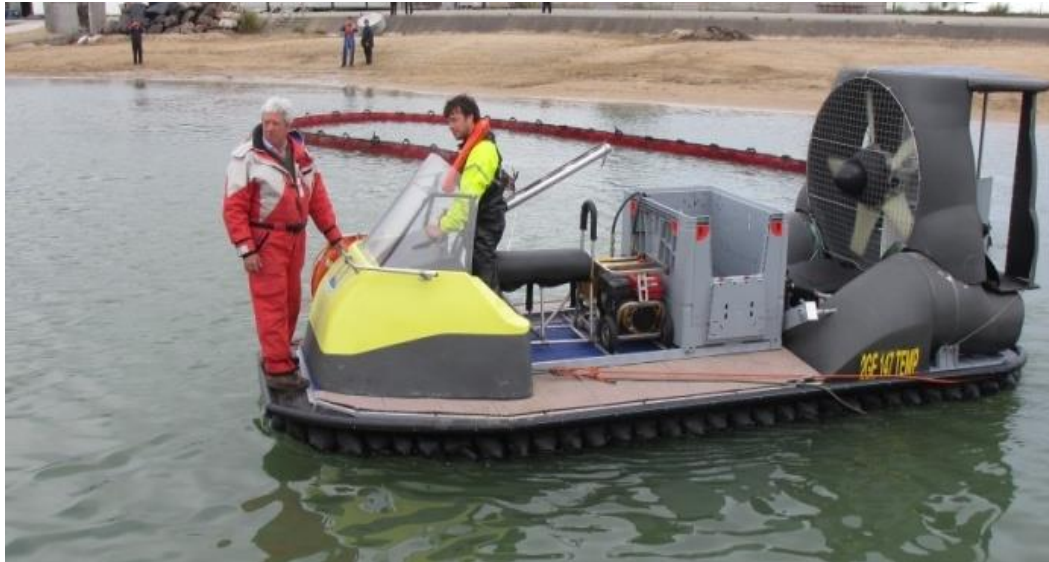
FIGURE 1. HOVERSPILL™ PLATFORM (DEVELOPED BY HOVERTECH) TO BE EQUIPPED WITH TURBYLEC SEPARATOR.
