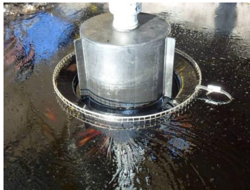
FIGURE 6. MECHANICAL SELF-ADJUSTING WEIR SKIMMER IN OPERATION.
