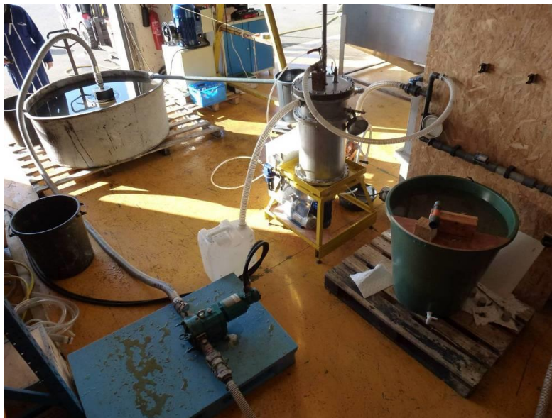
Figure 5. Turbylec: tests at Cedre (Demi Terrapin skimmer in a tank with oil, Börger A25 pump and Turbylec separator)
